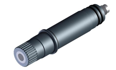
The WaterTechw<sup>2</sup> pH8000 Sensor has been designed to provide highly reliable pH and Temperature measurements. The sensor uses a flat surfaced electrode which includes an extended reference path, these features combine to provide an extremely robust pH measurement, suitable for use in surface water, wastewater and drinking water applications.
