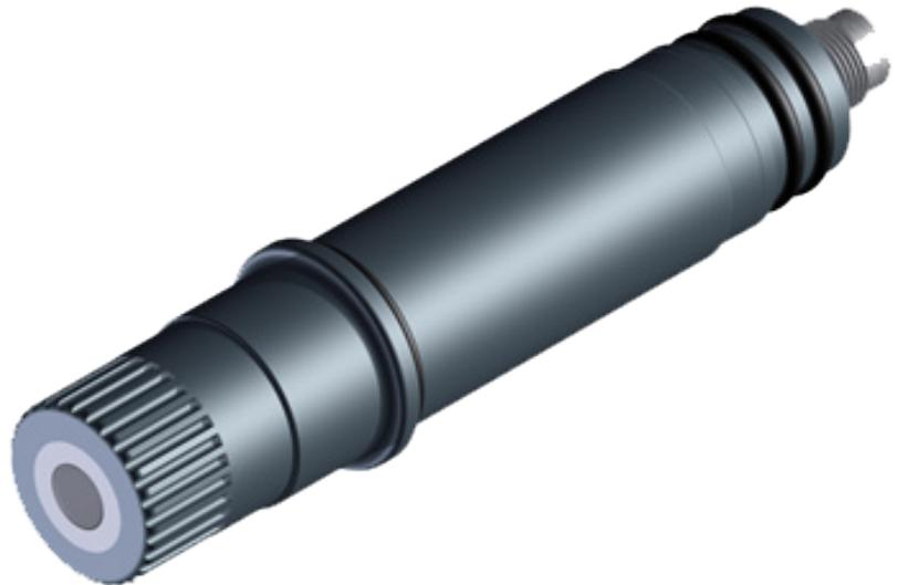
The WaterTechw<sup>2</sup> pH8000 Sensor has been designed to provide highly reliable pH and Temperature measurements. The sensor uses a flat surfaced electrode which includes an extended reference path, these features combine to provide an extremely robust pH measurement, suitable for use in surface water, wastewater and drinking water applications.
